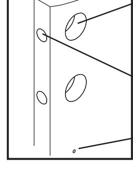
Drill 2-1/8" holes on door face from both sides to avoid wood splitting.
