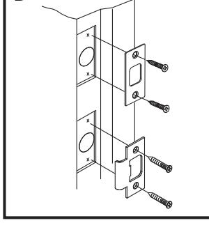
a. Match screw holes on strike with vertical centerlines on jamb. Mark outline of strike plate and chisel out until strike is flush with jamb. (Approx. 1/8")
