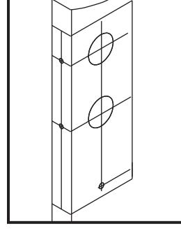
Select 2-3/8" or 2-3/4" backset as desired and mark center of holes on door face.
