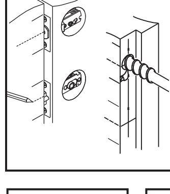
Measure one half of door thickness from doorstop and mark for the vertical centerline of strike. Drill 1" hole, 1/2" deep at the intersection of the horizontal and vertical centerlines.
