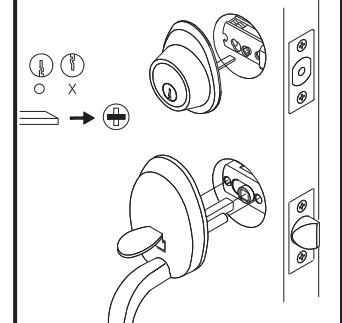
Retract deadbolt to unlocked position. Insert deadbolt cylinder in decorative trim and insert tailpiece horizontally through deadbolt latch hole. Place exterior handle with stems and square spindle into latch as shown. Press tightly against door face.
