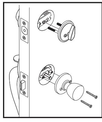
**Deadbolt:** Press cylinder side flush against door making certain the torque blade is properly positioned in latch crank. Tapped holes in housing of exterior cylinder should be lined up with screw holes. Key should be in down position.
