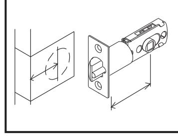
Backset is the distance from the door edge to the center of the hole on the door face. Master Lock door locks are supplied with an adjustable latch which can fit 2-3/8" or 2-3/4" backset.
