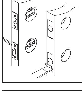
Insert latch in hole, mark outline of face plate and chisel 11/64" deep.
