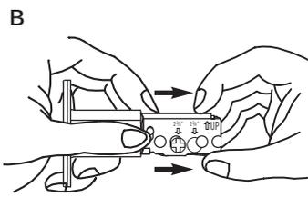
b. Push the change lever up against the top. Hold torque plate and torque spring then pull the extension plate all the way out. Be sure the 2-3/4" (70mm) screw hole is properly aligned and "change lever" jumps down to original position.
