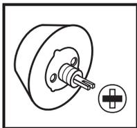
Press exterior cylinder flush against door. Exterior torque blade should be horizontally inserted into latch crank first.
