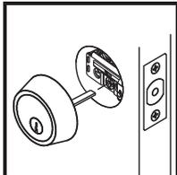
Press cylinder side flush against door making certain the torque blade is properly positioned in latch crank. Tapped holes in housing of exterior cylinder should be lined up with screwholes.
