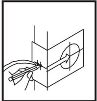
Select 2-3/8" or 2-3/4" (60mm or 70mm) backset as desired and mark center of hole on door face.
