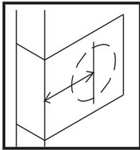
Backset is the distance from the door edge to the center of the hole on the door face. Master Lock door locks are supplied with an adjustable latch which can fit 2-3/8" (60mm) or 2-3/4" (70mm) backset.
