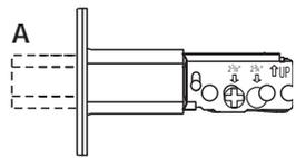
a. Rotate latch crank to retract the latchbolt to the unlock position.
