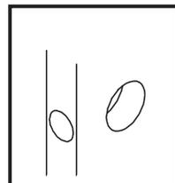
Drill 2-1/8" (54mm) hole on door face from both sides to avoid wood splitting. Drill 1" (25.4mm) hole for latch.
