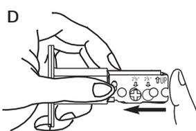
d. Latch may be adjusted back to 2-3/8" (60mm) backset by retracting the latchbolt, pushing up the "change lever" and moving the extension plate back to its original position.
