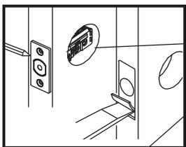
Insert latch in hole, mark outline of face plate and chisel 11/64" (4mm) deep.
