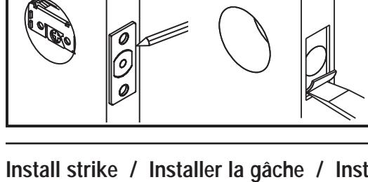
Insert latch in hole, mark outline of face plate and chisel 11/64" deep.
