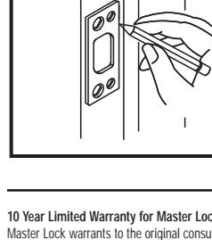
Match screw holes on strike with vertical centerlines on jamb. Mark outline of strike plate and chisel out until strike is flush with jamb. (Approx. 5/64")
