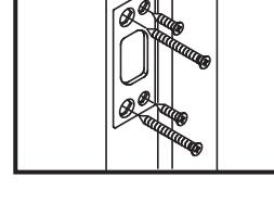
Install strike and tighten screws.
