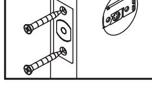
Insert latch and tighten screws.
