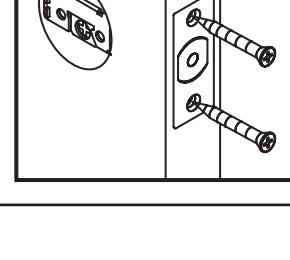
Insert latch and tighten screws.
