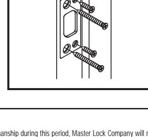
Install strike and tighten screws.
