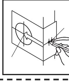
Select 2-3/8" or 2-3/4" backset as desired and mark center of holes on door face.
