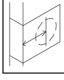
Backset is the distance from the door edge to the center of the hole on the door face. Master Lock commercial deadbolts are supplied with a 2-3/8" to 2-3/4" backset.
