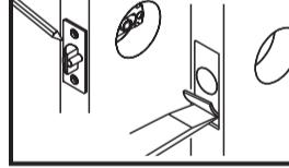
Insert latch in hole, mark outline of face plate and chisel 11/64" (4mm) deep.
