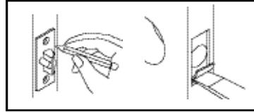
Insert latch in hole, mark outline of face plate and chisel 1/8" deep.
