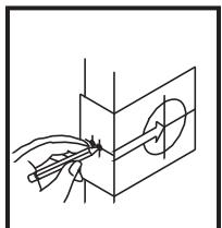
Backset is the distance from the door edge to the center of the hole on the door face. Master Lock door locks are supplied with an adjustable latch which can fit 2-3/8" (60mm) or 2-3/4" (70mm) backset.
