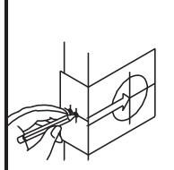
Select 2-3/8" or 2-3/4" (60mm or 70mm) backset as desired and mark center of hole on door face.
