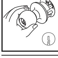
Insert spindle through latch. Press flush against door. (NOTE: Key hole must be in down position).
