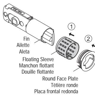
Locate floating sleeve and round face plate and proceed.
