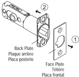
1. Use a flat screwdriver to separate the face plate.
