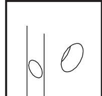
Drill 2-1/8" (54mm) hole on door face from both sides to avoid wood splitting. Drill 1" (25.4mm) hole for latch.
