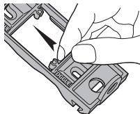
To change between "TOGGLE" and "ROCKER", apply firm pressure to remove the Dual Purpose Slide from Base. Flip the Slide over and snap back into place. Repeat on second Slide.
