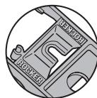
When "ROCKER" appears through the cover, the lockout device is set for a Rocker or Paddle style switch.
