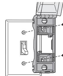
Loosen or remove screws.
