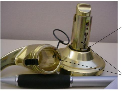
Tool presses spring loaded retainer clip
